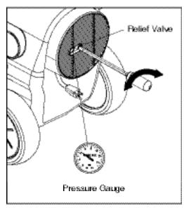
Figure 19. Adjusting Pump Pressure
